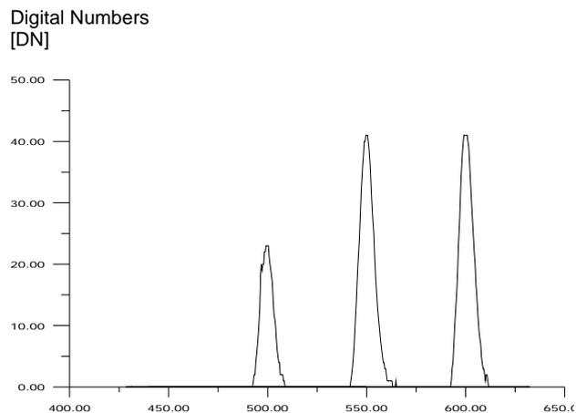
Fig. 4. Determination of the spectral range. Instrument's response to input impacts with central wavelengths  $\lambda_0$  of 500nm, 550nm and 600nm
