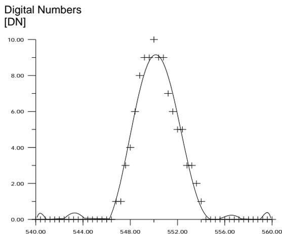
Fig. 3. Spectral response function for the 550nm channel (polynomial approximation) of a videospectrometer ( $\Delta\lambda_{in} 1.65\text{nm}$ )
